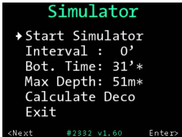
Use the simulator to simulate the dive mode of the OSTC 2 or to calculate the decoplan for your next dive. Using the simulator you can get familiar with your dive computer even before the first dive.
