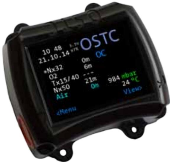
heinrichs weikamp delivers the OSTC 2 ready for use with a high quality rechargeable lithium battery. Anyway we recommend to load the OSTC 2 completely before you use it the first time.
